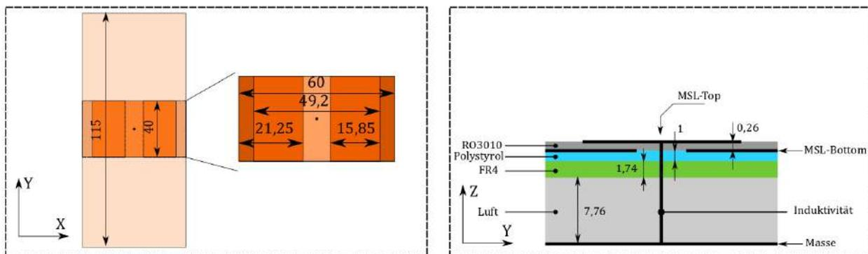
Fig. 1: (left) Top view and (right) side view of the designed UC; all the measures are given in mm.
