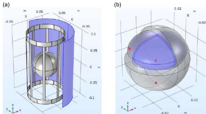
Fig. 1: (a) Birdcage coil geometry, EM shield and the phantom placed in the center of the coil. (b) Phantom geometry. The blue tissue (region c) is the brain tissue, region b is bone tissue equivalent and region a is filled with muscle.
