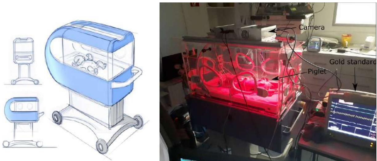
*Fig.1: Left: Schematic representation of the project objective incubator. Right: Proof of Concept Incubator at a piglet measurement series at the University Hospital in Homburg.*
