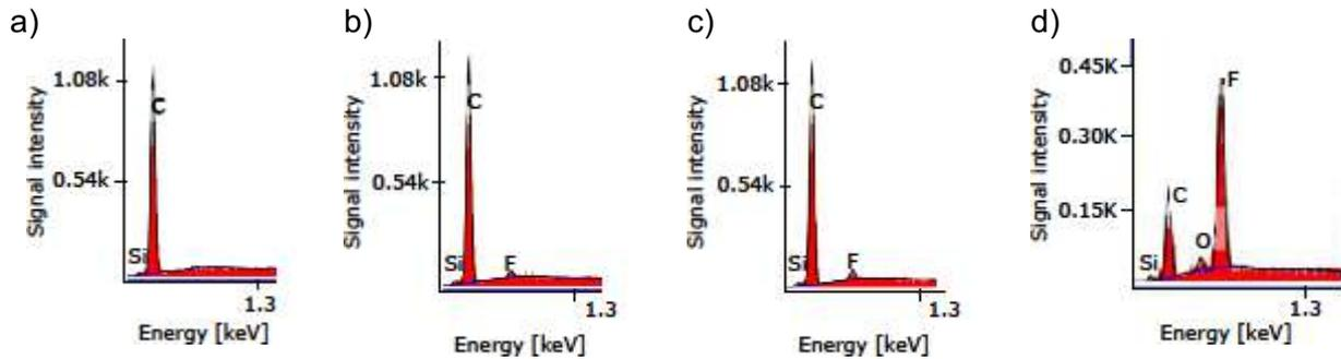
Fig.2: Measurement result of the energy dispersive X-ray spectroscopy of (a) DLC, (b) DLC fluorinated in SF<sub>6</sub>-plasma, (c) DLC deposited with C<sub>4</sub>F<sub>8</sub> and (d) Si deposited with C<sub>4</sub>F<sub>8</sub>.
