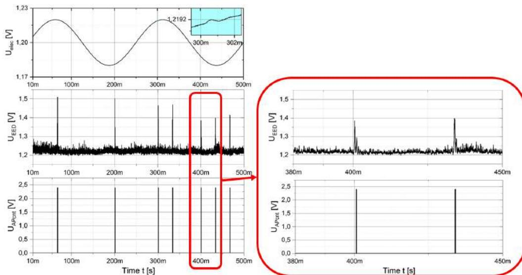
Fig.2: left: Transient noise simulation of the presented recording channel, with the electrode voltage at the input stage  $U_{elec}$ , the output of the spike detection  $U_{EED}$  and the detected spike for the digital counter  $U_{APcnt}$  – right: Enlargement of the time period from 380 ms and 450 ms.
