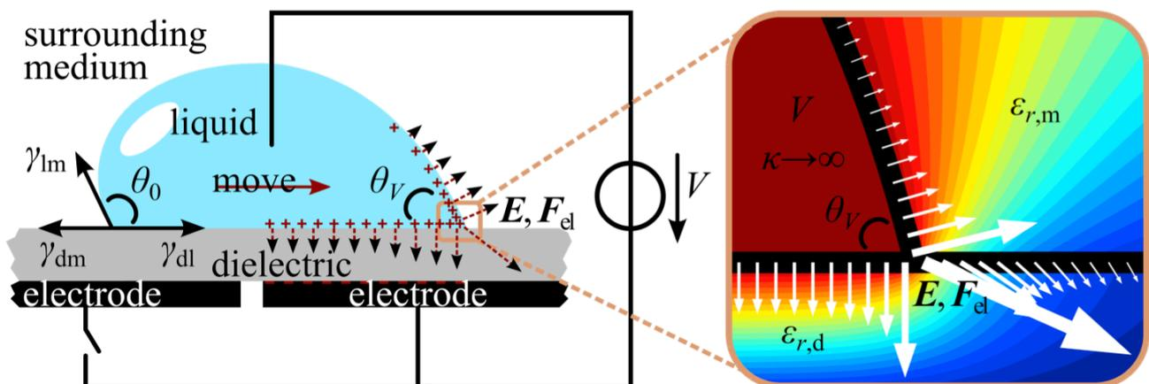
Fig.1: Scheme of the droplet transport between two electrodes. When the right electrode is activated, the estimated electric forces concentrate in the vicinity of the right-hand triple point of the perfectly conductive droplet. This specific asymmetric distribution of forces causes the directed motion of the droplet with the decreased right contact angle.
