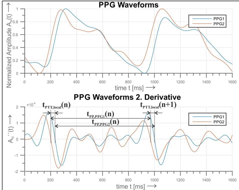
Fig. 1: PPG Waveforms measured by two sensors in a short distance (upper graph). Second derivative of the waveforms and derivable parameters (lower graph).
