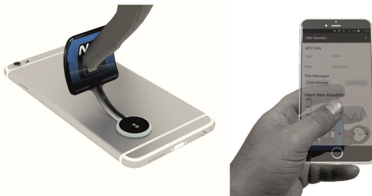
Fig. 1: Visualization of the sensor patch. Attachment of the patch on the backside of the smartphone (left). Execution of measurement while using the smartphone (right).
