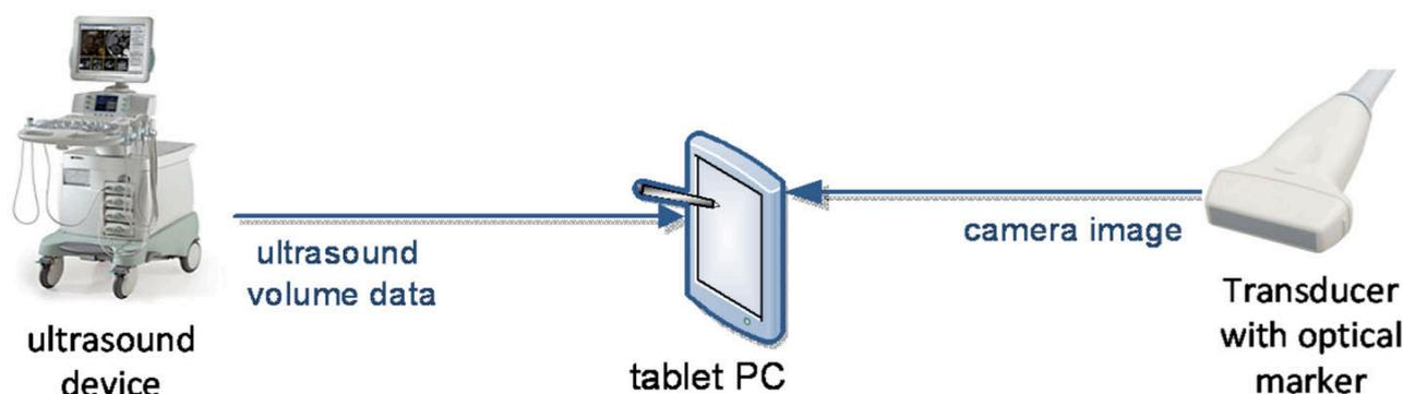
Fig. 1: Data flow for realizing AR ultrasound on tablet PCs
